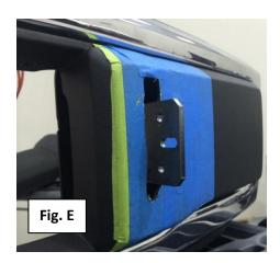
**<u>Step 7</u>**: Install Light bar/Pre-Runner to the bumper brackets using the supplied M6x20mm, M6 flange nuts and M6 washers and leave loose.
