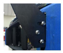
**<u>Step 8</u>**: After Light bar/Pre-runner has been properly adjusted, tighten all hardware. Your install is now complete.
