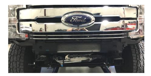
**6.** Remove the (x2) tow hooks and set aside.
