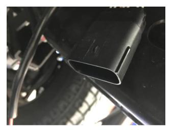
**2.** If equipped, unplug the block heater plug located on the passenger side inner frame horn. Remove plug from bumper. Plug back together and secure out of the way.
