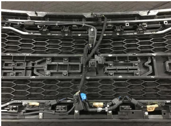
**14.** Re-install the shutter assembly back to your grill. Be sure all the electrical connections inside the grill are plugged back in before it is completely secured.
