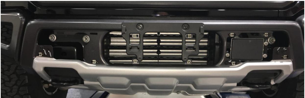
2. Remove the x3 nuts holding the Adaptive Cruise Control module on the studs.
