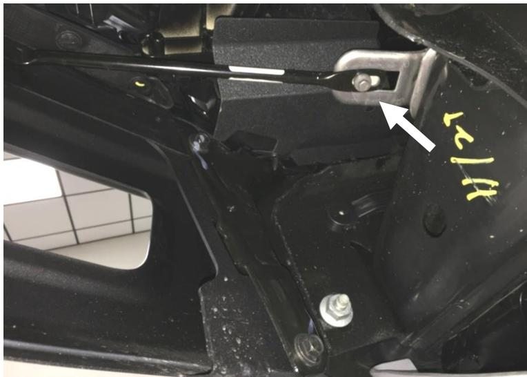
6. Remove the 21mm nuts that hold the bumper. There will be two per side that can be reached from the front and one on both sides that is accessible from behind the bumper.
