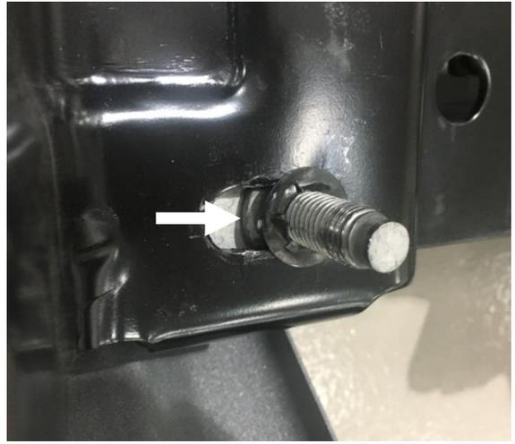
8. Remove the two bolts that hold the inner cooler cross brace,
