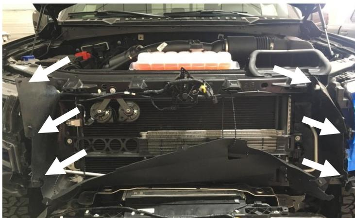
8. Remove the lower bolt that attaches the grill to the core support. (Bothe sides)
