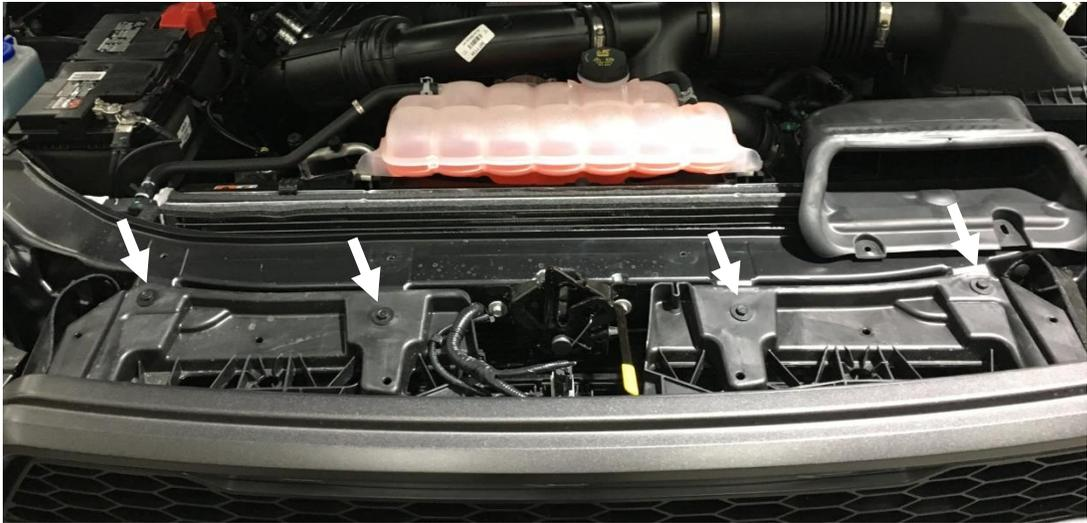
3. Remove the push pin that attaches the head light bezel to the core support.
