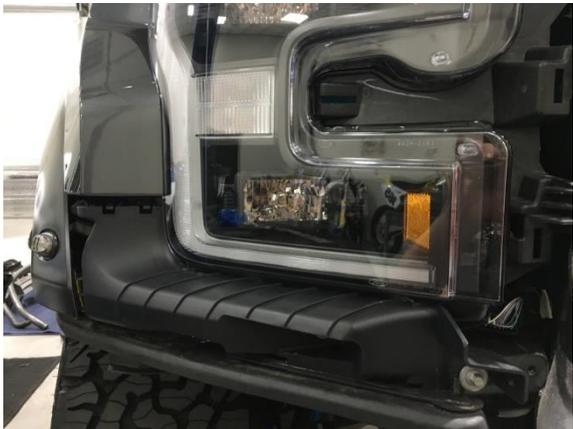
5. Unplug the two electrical connectors and undo the water line that is under the radiator cover.
