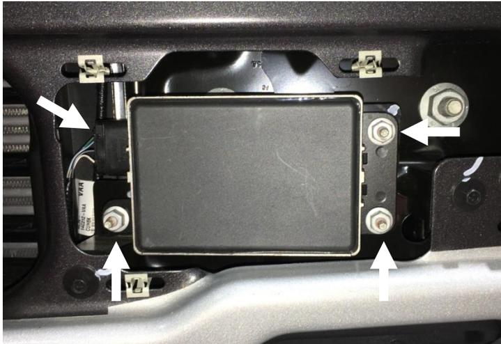
5. Remove the 8mm bolt that attaches the support bar to the bumper. (Bothe sides)
