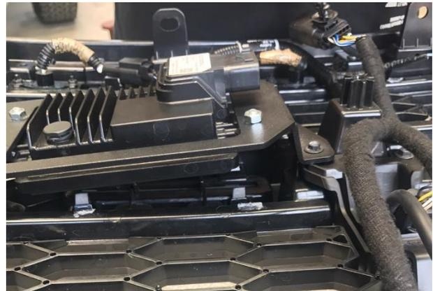
**12.** Using a 1 ½" hole saw, drill a hole in the bottom of your grill for the module harness plug to pass through.
