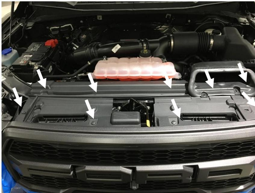
2. Remove the x4 bolts that attach the grill to the core support.
