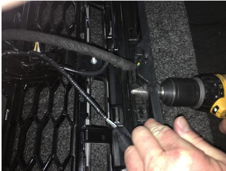
**13.** Add a couple of zip ties to secure the harnesses to the center of your grill making sure the module harness connector is accessible through the hole you drilled.
