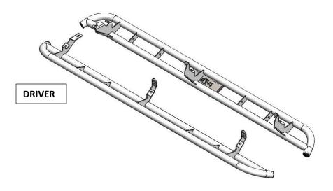
**STEP 2:** Remove any factory running boards or hardware and discard. **STEP 3:** Clean/tap the three factory threaded mounting locations.
