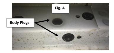
**Step 4:** Using the measurement from the brackets, only remove the rubber plugs from the sections you will need to mount the step. (**NOTE**: Start with the first section nearest to the front of the vehicle.)
