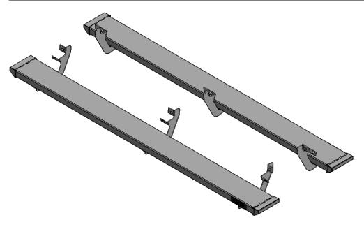
**Step 1:** Beginning with the driver side, remove any factory running boards or steps and discard.
