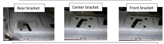
U-clip positioning. NOTE: Clip orientation will be the same for passenger side.
