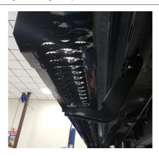
**Step 6:** Insert the supplied threaded bracket (x3) inside the running board lip over the top of each bracket.
