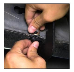
**Step 6:** Tighten pinch weld mounts first then upper bolts. Tighten to 20 ft./lbs. torque to secure the steps to vehicle.
