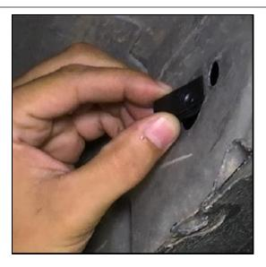
**Step 4:** Carefully place step into place. Use bolt, washer and begin hand tightening all three upper mounts. An assistant recommended with this step.
