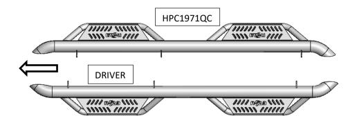
**Step 2** Install the (x6) mounting brackets to each attachment point on the main tube and leave loose for now.
