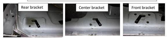
U-clip positioning. *NOTE: Clip orientation will be the same for passenger side.*
