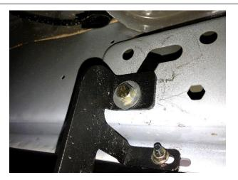
**<u>Step 11.</u>** After finial adjustment, tighten all three brackets at the main tube.
