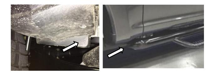
**Step 6.** Starting with the rear bracket, push up towards the pinch weld so the 3" main tube is high and tight to the body of the vehicle and use the supplied M8 nut, m8 hex bolt and washers to secure the bottom stud first.
