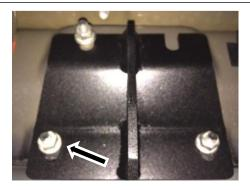
**<u>Step 8.</u>** After finial adjustment, tighten all four brackets at the main tube.
