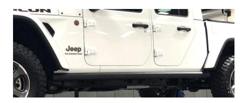
**Step 4.** Carefully raise step up into position and align the brackets with the factory mounting points with the horizontal part of the bracket on the outside of the pinch weld.
