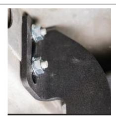
**Step 7.** After finial adjustment, tighten all three brackets at the main tube.
