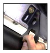
Step 6: Tighten to 20ft/lb torque to secure the steps to the vehicle.
