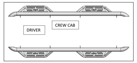
Step 2: Install the (x6) mounting brackets to each attachment point on the main tube using the supplied M10x25 carriage bolts, M10 hex nuts and leave loose for now. \*\*\*\* NOTE: The brackets will attach to the backside of the mounting flange with the threaded end of the carriage bolt facing towards the REAR of the step. \*\*\*
