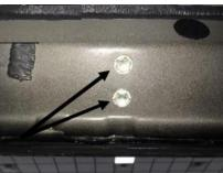
**Step 4:** Position step up to the body of the vehicle and align the brackets up with the factory mounting locations.
