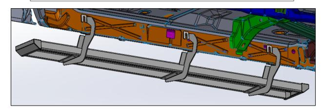
**Step 5:** Insert the supplied threaded brackets (x3) inside the running board lip over the top of each bracket.
