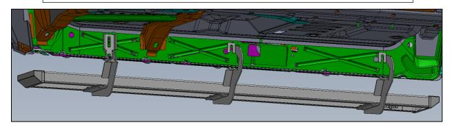
**Step 6:** Insert the supplied threaded brackets (x3) inside the running board lip over the top of each bracket.
