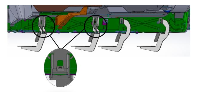
12302 Shiloh Church Rd. Houston TX 77066 REVISION -- © 2018 N-FAB, INC. Phone (281) 880-6322 - Fax (281) 880-6325 REVISION DATE 11/08/19 **<u>Step 6:</u>** Set running board along the top of all four brackets and center along the cab.
