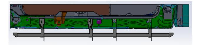
**<u>Step 7</u>**: Insert the supplied threaded brackets (x4) inside the running board lip over the top of each bracket.
