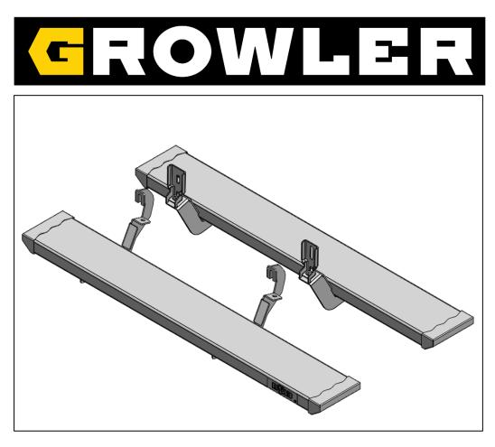
**Step 1**: Look on the underside of the body and locate the factory supplied mounting positions. **NOTE:** Some vehicles require the use of speed clips and nuts, which are supplied with the hardware kit.
