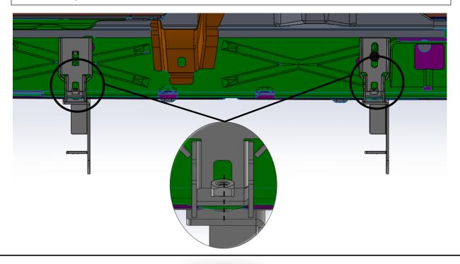
**<u>Step 6</u>**: Set running board along the top of both brackets and center along the cab. **<u>Step 7</u>**: Insert the supplied threaded brackets (x4) inside the running board lip over the top of each bracket.
