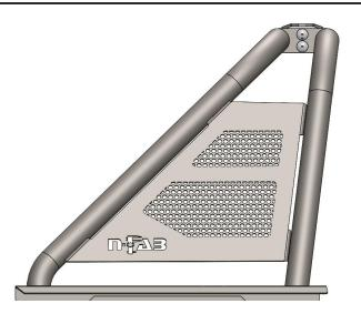
**Step 1**: Attach the Center section to the driver and passenger side assemblies using the supplied 3/8" x 1" carriage bolt (x4) and 3/8" fanged nut (x4) and leave finger tight for now. \*NOTE: Begin with the upper bolt and nut first to have easier access to the lower fasteners. \*
