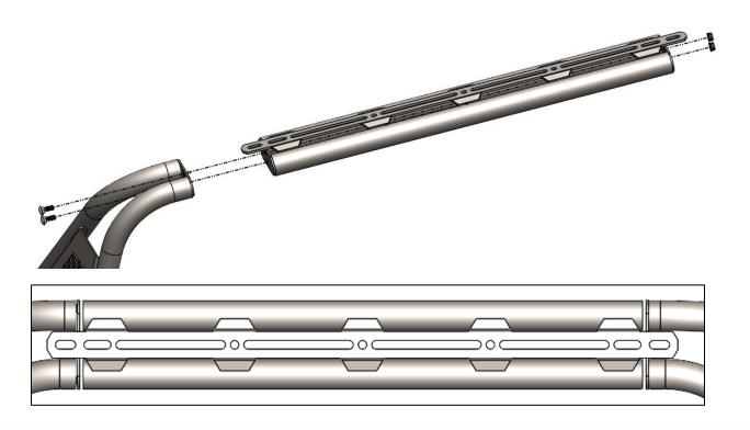
**Step 2:** With additional help, carefully place Sport Bar onto bed rails aligning edge with the plastic cap on both sides.
