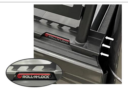
**<u>Step 3</u>**: Slide (x6) threaded channel nuts through rear opening of the T-slotted bed rail and align with the mounting holes in the Sport Bar.
