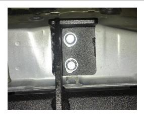
**<u>Step 4</u>** Start the remaining hardware with the front and rear bracket and leave loose.
