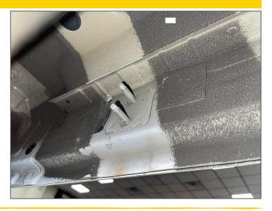
Step 3. Next, place (#1) Driver side step on the studs and secure with supplied (#3,#4) M8 flanged hex nut and M8 flat washer and loosely tighten for now.
