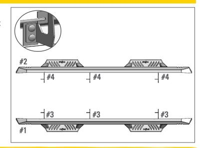
Step 3. Carefully raise (#1) driver side assembly up into position, aligning brackets with OE threaded studs and loosely secure with (#7)x6 M8 flanged hex nut.
