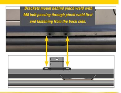
Step 8. After finial adjustment, tighten the (x3) upper mounts.
