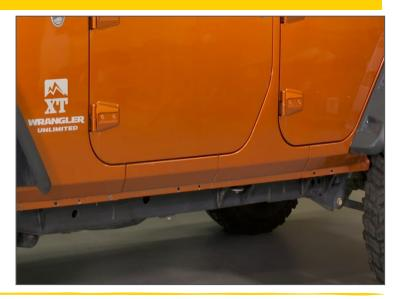
Step 2. Locate the (x3) factory mounting location on the pinch weld. Each location will have (x2) 3/8" holes. Step 3. Depending on the year of your vehicle, you may need to open up the holes using a 3/8" drill bit. Complete this step at this time.
