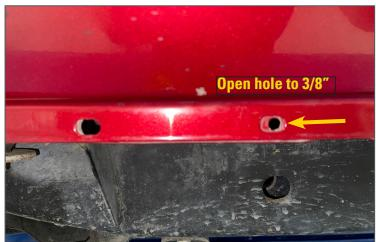
Step 4. Locate the (x3) mounting locations on the underneath of the floor pan. Depending on the year, you may have M8 threaded holes or slots for U-clips.
