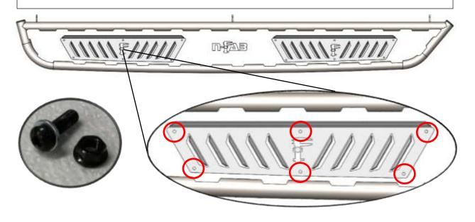
**Step 3:** Install (x3) mounting brackets to each attachment point with the supplied 3/8"x1" carriage bolt and flanged 3/8" nut on the main tube. Hand tighten for now. Repeat with passenger side.
