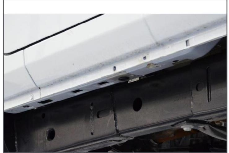
**Step 2. Carefully raise up (#1) driver side rail into position and align the brackets with the factory mounting points with the horizontal part of the bracket on the outside of the pinch weld.**
