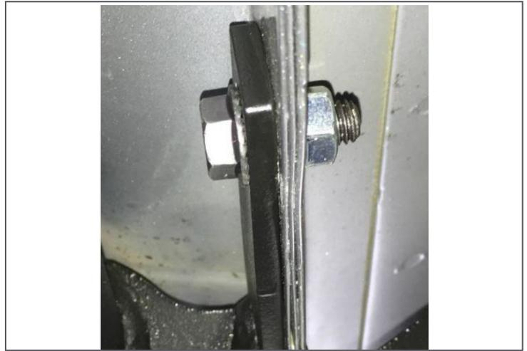
**Step 7. Next, tighten the remaining hardware that attaches the bracket to the upper body mount. (15-20 ft/lbs)**
