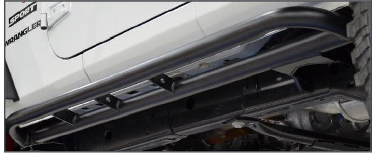
**Step 6. First, tighten all hardware that attaches the bracket to the pinch weld of the vehicle. (15-20 ft/lbs)**
