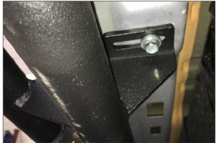
**Step 4. Start two (#4) M8x25mm black zinc flanged bolts and two (#5) M8 flanged nuts (both brackets) in the pinch weld and leave loose for final adjustment.**
