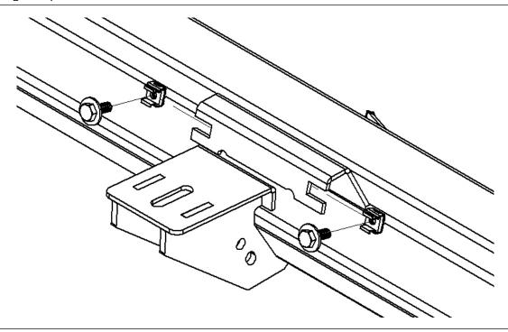
**Step. 7** After finial positioning, tighten all (x6) ¼"x ¾" hex bolts no more than 6 ft/lbs. torque.
