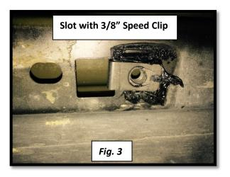
**Step. 3** Starting with the passenger side step rail, install the supplied (x6) ¼" snap nuts into the two notches in each mounting bracket.
