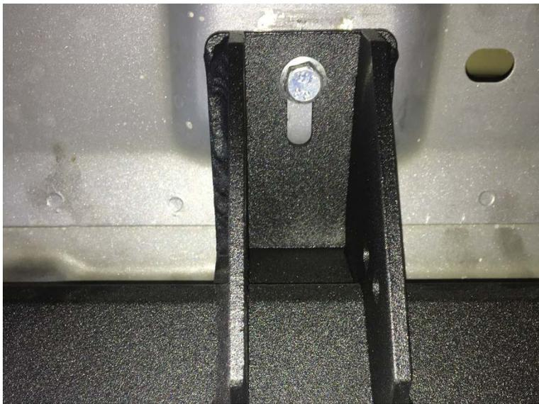
**Step.5.** Next, go ahead and install the two remaining M8x30mm hex bolts in the upper mounts and leave loose at this time.
