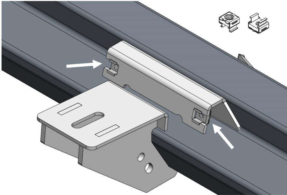
**Step.3** Carefully raise step rail up to the pinch weld of the body and align brackets up with the factory mounting locations.
