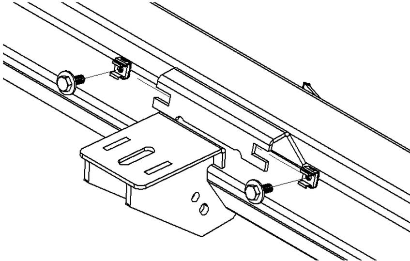
**Step. 7** After final positioning, tighten all (x6) 5/16 "x 3/4" hex bolts no more than 6 ft/lbs. torque.
