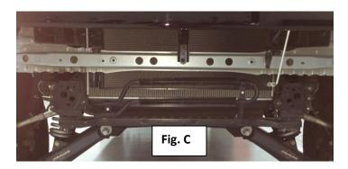
**Step 4:** Install MRDS bumper to factory mounting studs and loosely fasten with the 14mm hex nuts that were removed step 2.
