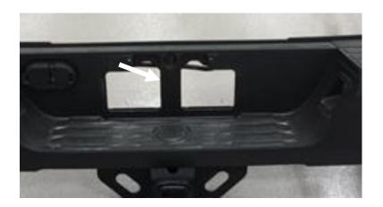
**Step 5:** Remove the plastic end cap. (Both sides)
