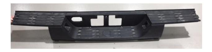
**Step 7:** Remove the four top bolts and two lower bolts that attach the bumper end and Remove. (Both sides)
