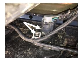
**Step 3:** Remove the license plate bulbs from there housing and secure up out of the way.
