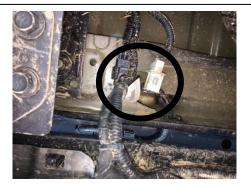
**Step 2:** Unplug the connecter on the back of the trailer light plug. Pres the two metal tabs together and push it out of the front of bumper.
