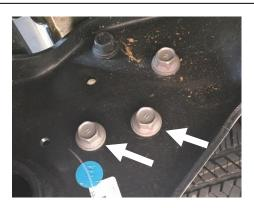
Step 2: Remove the two bolts that attach the OE bumper bracket and remove (Bothe sides))
