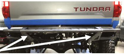
**Step 2:** After proper alignment, tighten all hardware. *NOTE: Carefully open tail gate to check clearance with bumper before final tightening.*
