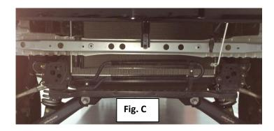
**Step 4:** Install MRDS bumper to factory mounting studs and loosely fasten with the 14mm hex nuts that were removed step 2.
