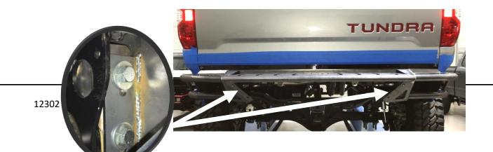
**Step 2:** After proper alignment, tighten all hardware. *NOTE: Carefully open tail gate to check clearance with bumper before final tightening.*
