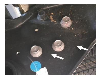
Step 2: Remove the two bolts that attach the OE bumper bracket and remove (Bothe sides))
