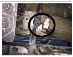
**Step 2:** Unplug the connecter on the back of the trailer light plug. Pres the two metal tabs together and push it out of the front of bumper.
