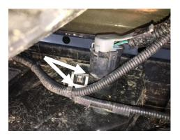
Step 3: Remove the license plate bulbs from there housing and secure up out of the way.
