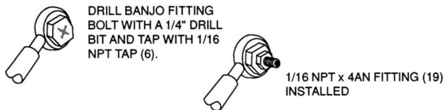
Figure 13 Schematic of “Drilled Out” Banjo Fitting
