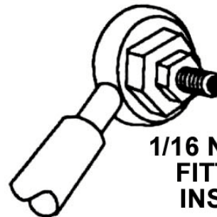
Figure 8 Schematic of "Drilled Out" Banjo Fitting
