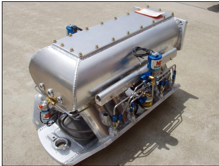
Figure 3 Typical Dry Dual Stage kit installed—Single Plane or Tunnel Ram Intake
