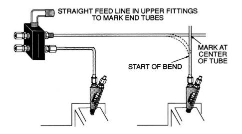
16. Remove the two nitrous solenoid extension tubes. Cut off the tubes at the inside end of the marks. Deburr and ream the cut ends.
