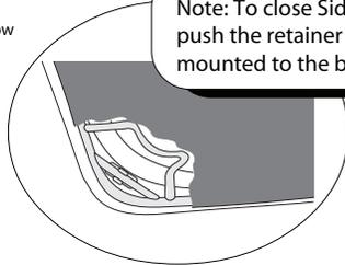
Rear Window Retainer Rod - Slide into sleeve
