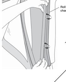
Roll Plastic Strip into channel in retainer
