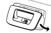
Tilt the bezel down, pull the handle as far as it will go out of the tailgate and slide the bezel over it. Push the bezel in until the spring clips snap into the tailgate. Insert the supplied 6 MM bolt in the center mounting hole and tighten (do not overtighten screw), then tighten the two 8 MM mounting bolts, making sure that the handle is straight.
