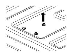
Lower the tailgate and remove the center 8 MM mounting bolt holding the handle and bezel.
