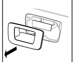
Close the tailgate and carefully pull the bezel away from the tailgate working against the three spring clips.
