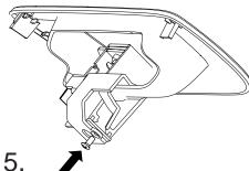
Turn the bezel around and insert the 6-32 screw as shown. Tighten it to secure the POP&LOCK in place making sure that it fits tightly in the corner of the bezel.
