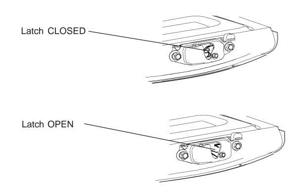
Insert screwdriver and push DOWN to CLOSE and install the PL1300.
