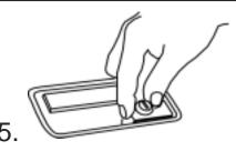
Now slide the POP&LOCK to the right so that the mounting bracket is positioned under the actuating rod on the passenger's side.
