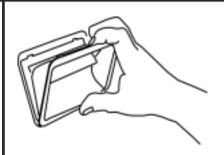
Remove the plastic insert by pivoting it on the bottom edge.
