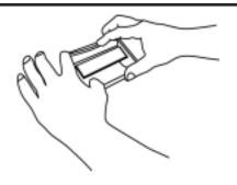
Carefully, squeeze the top edge of the black plastic insert down to release the top two locking tabs to prevent breakage.
