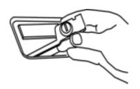
Insert the POP&LOCK bracket at an angle on the driver's side and push it all the way to the left to clear the passenger side actuating rod.
