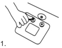
Loosen all three bolts of the handle. push the handle up as high as it will go and tighten the top bolt. Remove the bottom two bolts (see Fig. 7)
