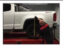
**STEP 2:** Position vehicle on a stable, flat surface or automotive lift. Be sure engine is turned OFF and vehicle is in PARK. Secure vehicle with wheel chocks.
