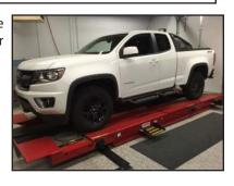
**STEP 3:** Raise the rear of the vehicle by the frame. Secure with jack stands.
