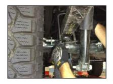
**STEP 7:** Lower axle to allow enough space for the new block kit to be installed.
