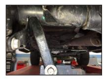
**STEP 5:** Remove the four U-bolt nuts and washers on each side of the vehicle, and remove lower U-bolt axle brackets.
