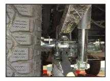
**STEP 6:** Remove OE U-bolts, and the lower shock fasteners, if required.
