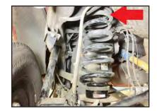
**STEP 12:** With vehicle all the way down. reconnect lower shock bolt and nut. Torque to manufacturer's specifications.
