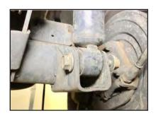
**STEP 13:** Reconnect rear sway bar links at each end of sway bar, and torque to manufacturer's specifications.
