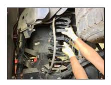
**STEP 11:** Slowly raise rear axle or lower vehicle onto the springs. Double check both upper isolators are fitting into their correct positions. Adjust accordingly.
