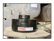
**STEP 10:** Reinstall OEM spring isolator on **TOP** of the block(s) and on **TOP** of spring. Make sure to seat the upper isolator correctly in it's original position.
