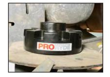
**STEP 9: 2.0" REAR LIFT OPTION.** Install both interlocking blocks combined.
