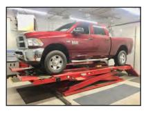
**STEP 2:** On a flat, level surface or automotive lift, MEASURE pre-installation ride height, FRONT & REAR, and write down measurements.
