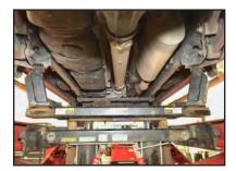
**STEP 6:** Remove coil spring and both upper and lower isolators.
