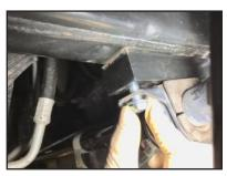
**STEP 7:** Reinstall sway bar end links and tighten to manufactuer's specs on both sides.
