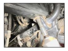
**STEP 5:** Install sway bar relocation bracket using OEM bolts on both sides.
