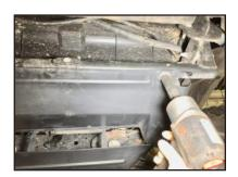
**STEP 3:** Remove sway bar links from both sides.
