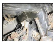
**STEP 6:** Lift sway bar back into place. Insert supplied bolts and washers on both sides.
