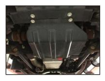
**STEP 3:** Locate the four axle mounting bolts. **Loosen the 21MM bolts but do not remove**, leave all top nuts a few threads on. Go slow as differential lowers.
