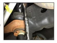
**STEP 5:** Start by removing one bolt at a time. Slide diff spacer between axle mount and frame mount.
