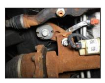
head ratchet with deep socket works the best. For the drivers side front use 21MM flex head wrench, stubby wrench or short adjustable wrench.
