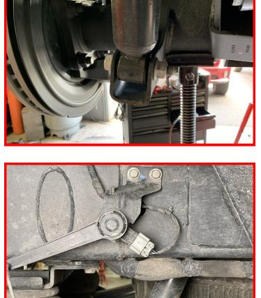
Plug the factory air suspension height sensors in.
