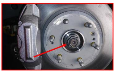
Remove brake caliper mounting bolts and hang caliper out of the way. Do not hang the caliper by the brake line. Retain factory hardware.
