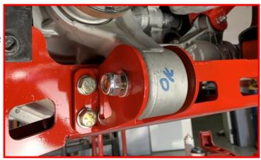
Tighten passenger differential drop bracket hardware.
