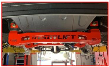
Using the supplied cam bolts, cams, washers and nuts, install the lower control arms in the factory orientation.
