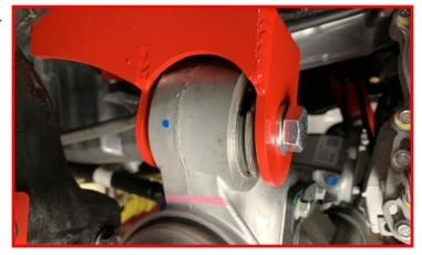
Tighten driver differential drop bracket hardware.
