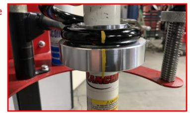
Install front strut spacers using factory nuts.
