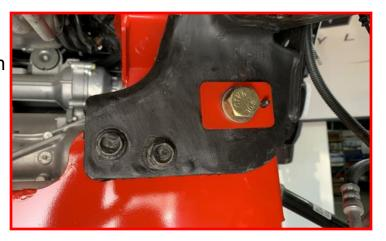
Install the (1) factory rear crossmember bolt and nut and supplied cam block off plates, M18 bolt, washers and nut through the driver side factory mount and replacement crossmember. Do not tighten hardware as this time.
