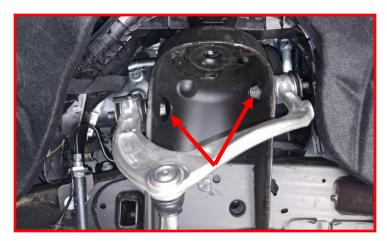
Remove (4) sway bar mounting bolts from the frame. Remove sway bar from the vehicle and retain factory hardware.
