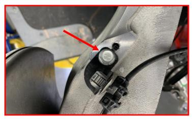
Remove the wheel speed sensor from the knuckle and hang out of the way. Retain the factory hardware.
