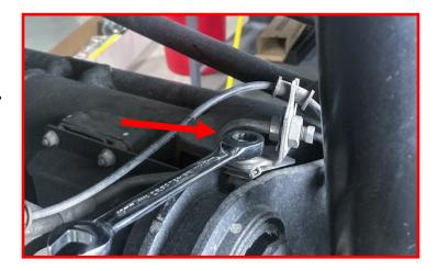
Remove the 13mm ABS and Brake line lower bracket bolt from the axle.
