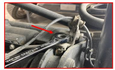
Loosen track bar bolts at the frame and axle ends.
