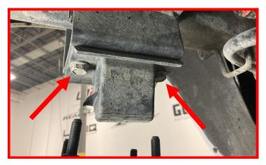
Install the provided bump stop extensions using the provided hardware.
