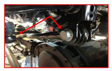
Loosen the rear radius arm bolt.
