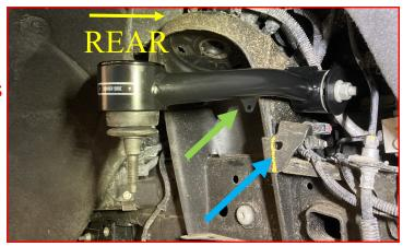
With the upper control arm bolts in place, install the supplied laser cut washers and oe nuts.
