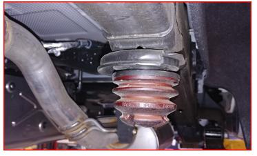
Install rear bump stop extension between frame rail and bump stop using supplied M10 Bolt.
