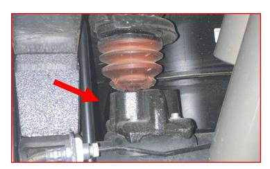
If the truck DOES NOT HAVE the 2" cast bump stop extension shown in the previous picture, INSTALL THE READYLIFT BUMPSTOP EXTENSION as follows.
