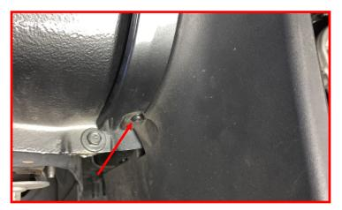
Peal back the fender trim to reveal two screw clips on the outer fender. Remove the lower clip holding the fender liner on.
