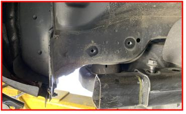
Remove the two factory M12 bolts and discard the cut factory beam.
