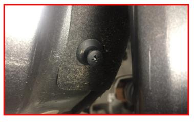
Install the factory T25 fender trim bolt. Tighten until snug.
