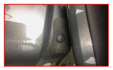
Carefully peal back the fender liner to reveal the four M8 bolts holding the plastic inner crash structure.
