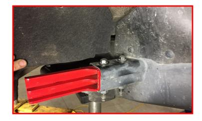
Using the factory hardware, install the plastic crash structure.
