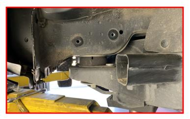
Install the replacement Rear Anti-Intrusion Beam using the factory hardware.
