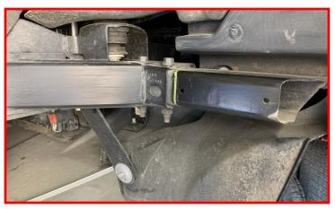
Remove the two factory M12 bolts and discard the cut factory beam.
