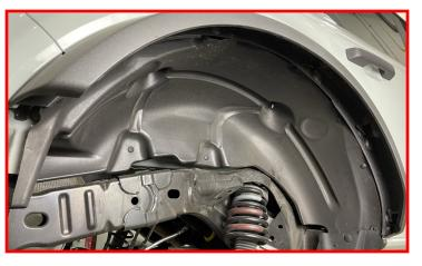
Remove the rear fender liners.
