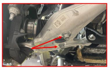
Loosen but do not remove the (2) forward sway bar skid plate bolts.
