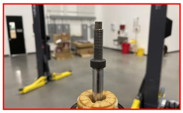
Remove the seal head bump cap.
