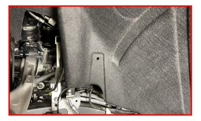
Install the driver and passenger rear sway bar retainer cap bolt.
