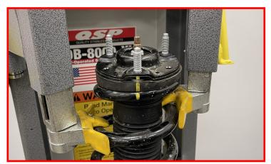
With the strut removed from the spring compressor, remove the factory strut shaft spacer.
