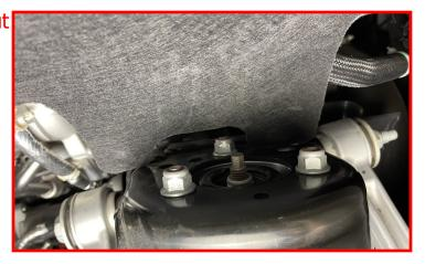
Remove the lower strut nuts.
