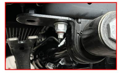
Lower the sway bar down and back to aid in removal of the rear lower control arm pivot bolt.
