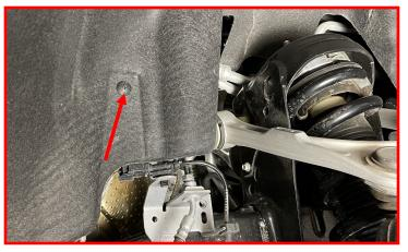
Remove the upper control arm heat shield mounting bolt. The heat shield is located on the rear pivot of the right (passenger) side on the vehicle.
