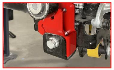
Install the supplied rear track bar bracket nut into the hole located in the factory track bar bracket.
