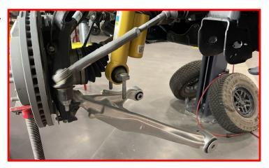
Remove the (3) top strut nuts and carefully remove the strut assembly from the vehicle.
