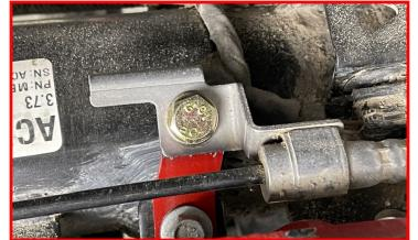
Install the rear track bar into the track bar bracket using the supplied M16 x 90mm hex head bolt, washers and locking nut.
