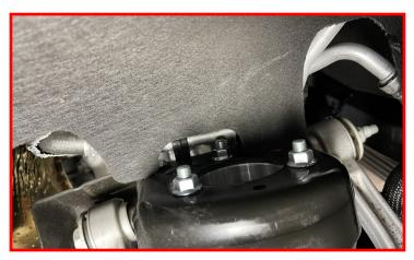
Remove the single retaining rivet that secures the inner fender liner.
