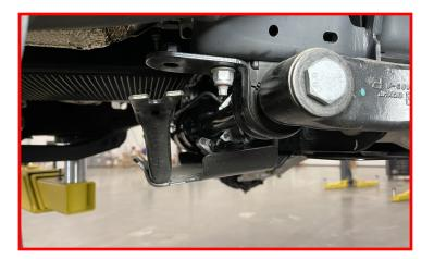
Remove both the driver and passenger forward sway bar retainer cap bolts.
