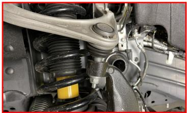
Remove the upper control arm pivot bolt.
