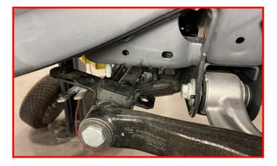
Install the driver and passenger rear sway bar retainer cap nuts.
