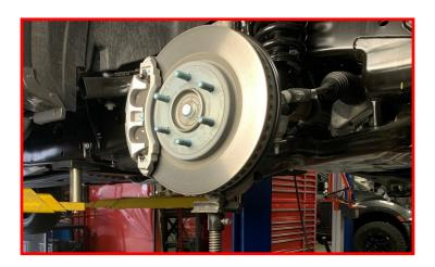
Remove the sway bar end link from the lower control arm.
