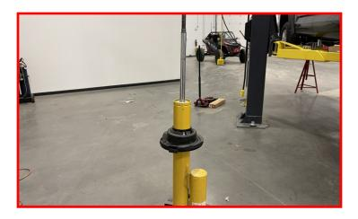
Install the seal head bump cap.
