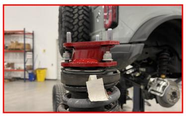
Using the supplied M10 nuts, install the completed strut assembly into the frame.
