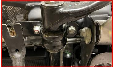
Remove both the driver and passenger rear sway bar retainer cap nuts.
