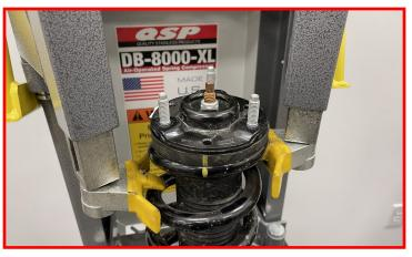
Before install the top strut spacer you will need to trim the factory top hat studs to make clearance for the strut spacer.
