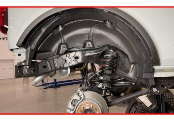
Prior to installing wheels, complete all installation steps on the opposite side. Install the wheels and lower the vehicle to the ground. Torque the lug nuts to the wheel manufacturers specs. Jounce the vehicle to settle the suspension to the new ride height.
