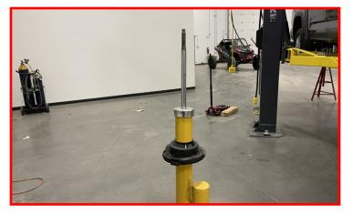
Install the factory bump stop and dust boot.
