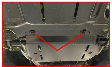
Remove both the driver and passenger rear sway bar skid plate bolts.
