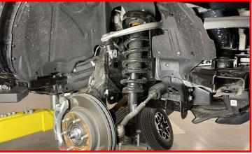
With the strut assembly removed from the vehicle, remove the locating pin from the top hat using pilers or similar tool.
