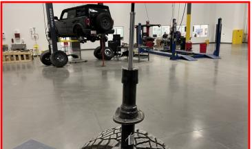
Before removing the spring perch, mark the orientation of perch to strut body. Ensure the mark is long enough to be visible once the preload spacer is installed.
