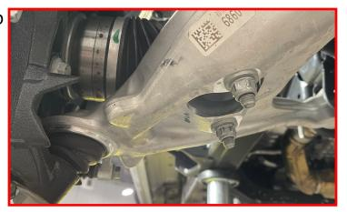
Using an appropriate jack, carefully jack the lower control arm into the frame side pivot pockets.
