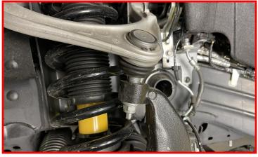
Remove the upper control arm pivot bolt.
