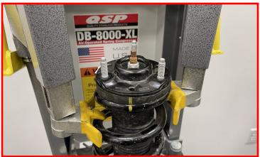
Install the top strut spacer onto the rear strut assembly using the factory nuts.
