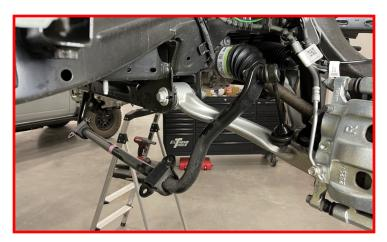
Install the sway bar end link into the lower control arm using the factory hardware.
