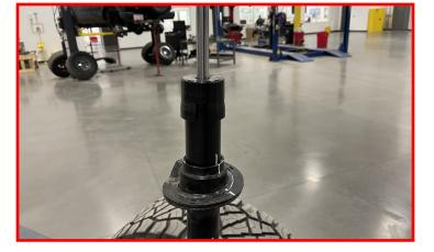
Install the factory bump stop and dust boot.
