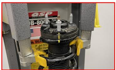
With the strut removed from the spring compressor, remove the factory bump stop and dust boot.
