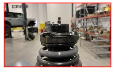
Place the strut into a spring compressor. Mark the top hat to spring location.
